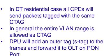
Later release will cater for enterprise customers that require multiple VLANs transparently forwarded with outer tag added
